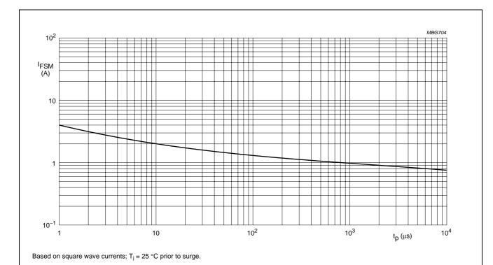
Fig.4 Maximum permissible non-repetitive peak forward current as a function of pulse duration per diode.
