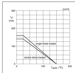
Device mounted on a FR4 printed-circuit board.
