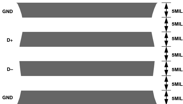
Figure 16. Typical Arrangement of Signal Tracks
