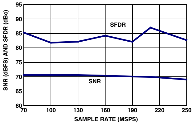
FIGURE 9. SNR AND SFDR vs f SAMPLE
