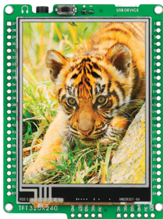
Figure 1: mikromedia for PIC32 development board
