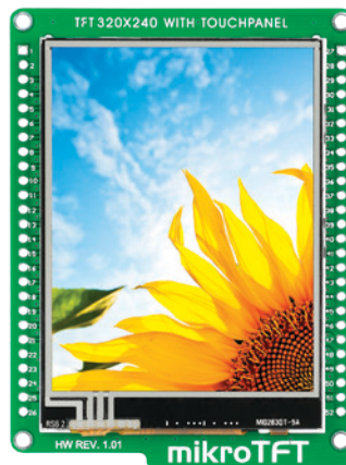
Figure 2: mikroTFT display board
