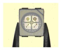
(3) When populating boards in SMT production, there are basically no restrictions regarding the form of the pick and place nozzle, except that mechanical pressure on the surface of the resin must be prevented.
