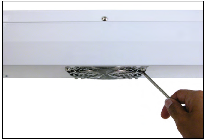
Figure 6. Shorting the ionizer's two fan grills
