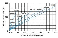
For resistor mounted on standard heatsink, related to power dissipation
