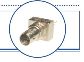
The OPF392 family fiber optic transmitters are high performance devices packaged for data communication links. This transmitter is an 850nm GaAlAs LED and is specifically designed to efficiently launch optical power into fibers ranging in size from 50/125µm up to 200/300µm diameter fiber. Multiple power ranges with upper and lower limits are offered which allows the designer to select a device best suited for the application.
