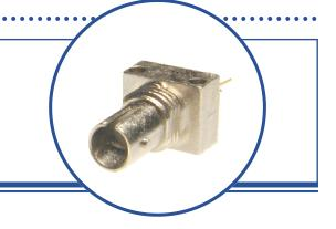
The OPF347 family fiber optic transmitters are high performance devices packaged for data communication links. This transmitter is an 850nm GaAlAs LED and is specifically designed to efficiently launch optical power into fibers ranging in size from 50/125µm up to 200/300µm diameter fiber. Multiple power ranges with upper and lower limits are offered which allows the designer to select a device best suited for the application.
