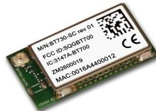
Every BT730 series Bluetooth® module from Laird Technologies is designed to add robust, long-range Bluetooth data connectivity to any device. Based on the market-leading Cambridge Silicon Radio (CSR) BC04 chipset, BT730 modules provide exceptionally low power consumption with outstanding Class 1 range via 18 dBm of transmit power. A broad range of Bluetooth profiles such as Serial Port Profile (SPP) and other vital features make BT730 modules superior to other Bluetooth modules.
