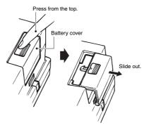
Pay careful attention to the polarity when inserting the battery. Insert the battery following the polarity marked in the battery box of the Time Switch. Before using the Time Switch, be sure to close the battery cover after the battery is inserted.
