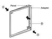
Once the adapter has been mounted, insert the Time Switch as illustrated at the right. Secure the Time Switch in two places using the enclosed screws (M3 x 16) tightened with a torque of 0.58 N·m max.
