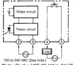
Note: On the H2F-30 (12 to 24 VDC), terminal number 2 is positive and terminal number 3 is negative.
