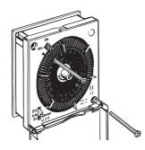
3. If the lead wire has been installed in front of the panel, place the Time Switch on part A of the adapter and push it in toward B. Then secure the Time Switch by tightening the screws as described in step 2.
