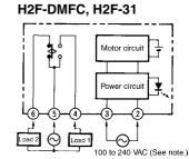
Note: On the H2F-31 (12 to 24 VDC), terminal number 2 is positive and terminal number 3 is negative.
