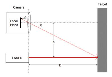
Referring to the figure, a laser diode module shines a laser spot onto the target object. The value h is a fixed, known distance between the center points of the laser diode and the camera (78 mm for the LRF Module). When the distance to the target object D changes, so do both the angle  $\theta$  and the value pfc (pixels from center), which is the number of pixels the centroid of the primary blob (laser spot) is away from the camera's center point.
