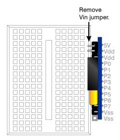
It is important to remove the Vin jumper from the DB-Expander board, unless you want your daughterboard's Vin pin to be powered by +5V.
