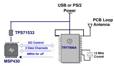
The TRF7900A simplifies system design by reducing system component count and manual circuit tuning. By integrating the PLL, SAW filter, and RF mixer, the TRF7900A eliminates the manual tuning of RLC circuits required in traditional implementations.
