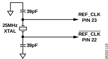
Figure 35. Crystal Input Configuration
