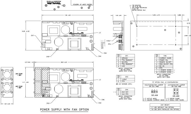
3 OPTIONAL-MOLEX CONNECTOR (OPTION 'K'-LIMITED TO 7A) MAY BE SPECIFIED FOR CNJ INSTEAD OF STANDARD OUTPUT STUDS.
