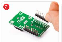
Turn the board upside down, so that bottom side is facing you upwards. Place shorter parts of the header pins in the both soldering pad locations.
