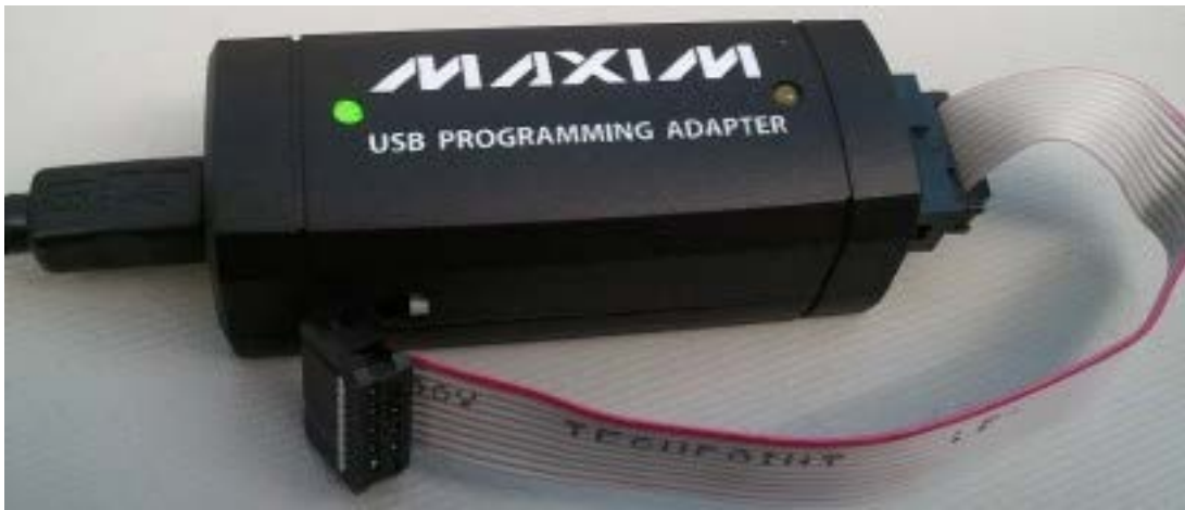
Figure 3. MAXQ USB-to-JTAG/1-Wire Adapter
