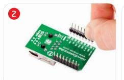
Turn the board upside down, so that bottom side is facing you upwards. Place shorter parts of the header pins in the both soldering pad locations.
