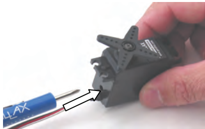
1) Insert tip of Phillips screwdriver into potentiometer access hole.
