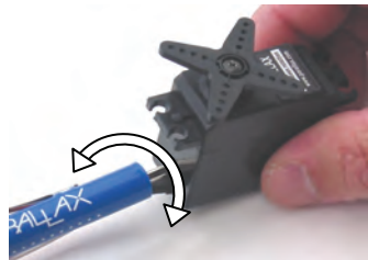
2) Gently turn screwdriver to adjust potentiometer until the servo stops moving.
