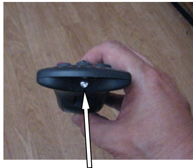
Figure 7-3: IR LED in a TV Remote Viewed through a Digital Camera
