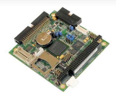
The TITAN is an ultra low power PC/104 compatible single board computer based on the 520MHz PXA270 XScale RISC processor. The PXA270 is an implementation of the ARM compliant, Intel XScale microarchitecture combined with a comprehensive set of integrated peripherals including: flat panel graphics controller, USB host/client controller, interrupt controller and multiple serial ports.
