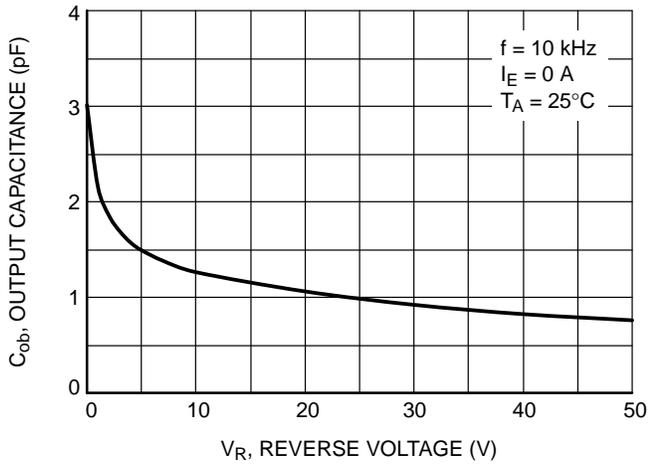
Figure 4. Output Capacitance
