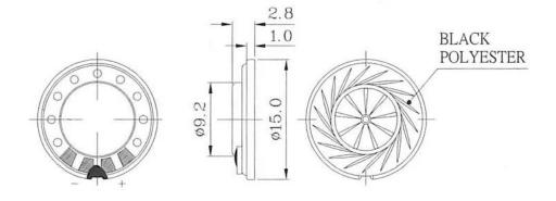
The mylar will not exceed the metal frame when input is at the maximum power of 0.5W.
