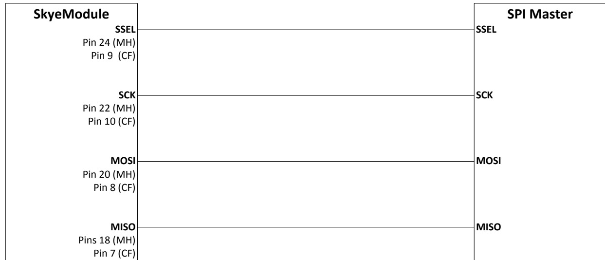
Figure 9-3: SPI Connection Diagram
