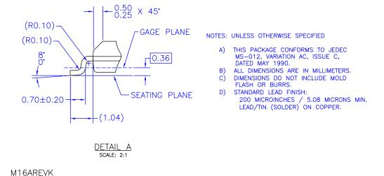
Figure 1. 16-Lead Small Outline Integrated Circuit (SOIC), JEDEC MS-012, 0.150" Narrow Package Number M16A
