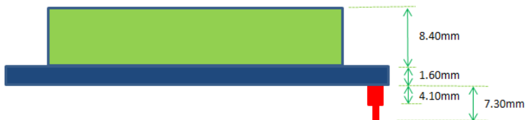
Figure 3-4 - VI800A-232U module PCB Side view
