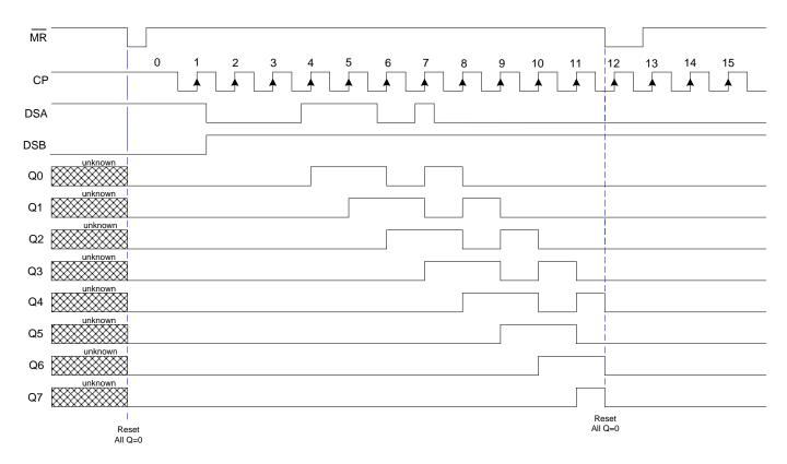
5. All Q values are reset to LOW when  $\overline{MR}$  goes low.  $\overline{MR}$  is asynchronous and overrides all other signals. 6. Serial data supplied at DSA and DSB is ANDED and transferred to Q0 on positive edge of CP. Notes:
