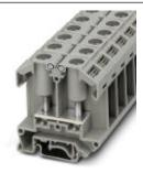
Universal terminal block with bolt connection, slotted-head screw, cross section: 1 - 25 mm², width: 18 mm, color: gray
