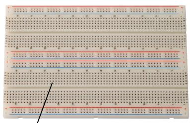
Move your completed project to a SB1660 Solderable PC BreadBoard
