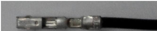
Fig.1: Showing female contact back side
