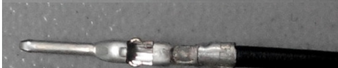
Fig.2: Showing male contact back side
