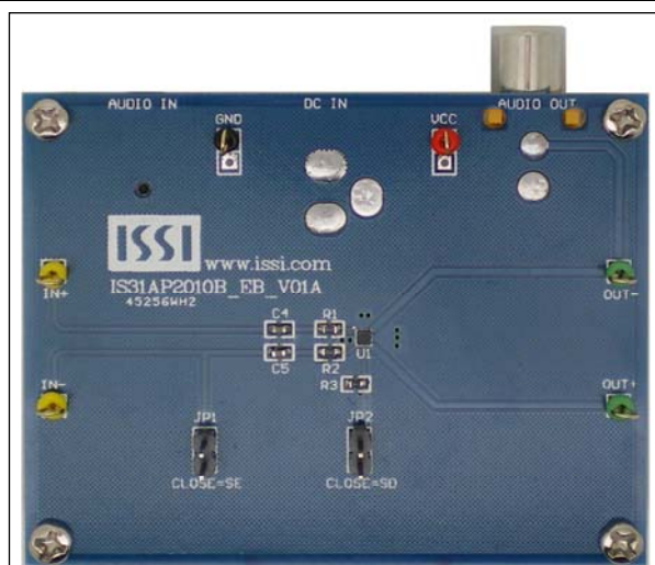
Figure 1: Photo of IS31AP2010B Evaluation Board
