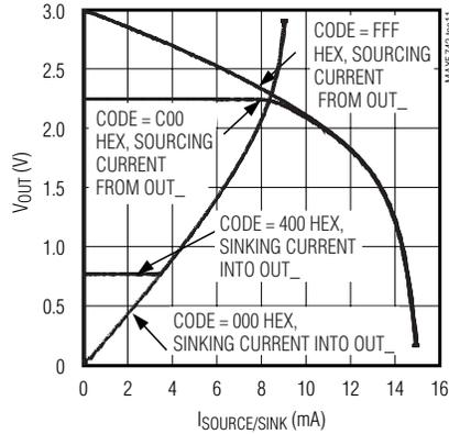
**SOURCE-AND-SINK CURRENT CAPABILITY ( $V_{DD} = +5V$ )**
