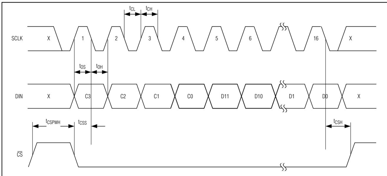
Figure 2. Timing Diagram
