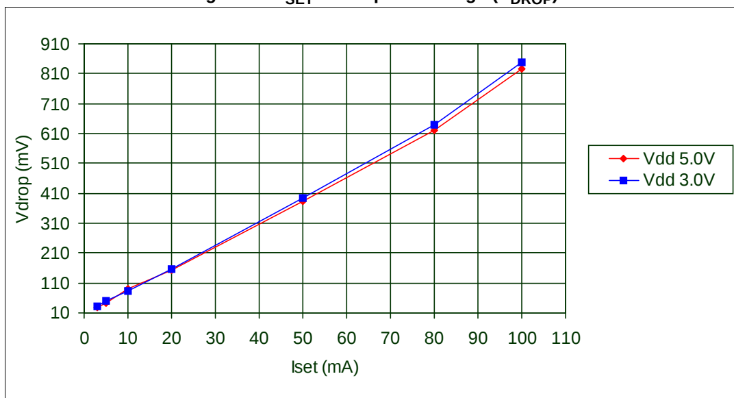
Figure 12. I_{SET} vs drop out voltage ( V_{DROP} )
