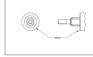
Shaft and panel seal switches are watertight to the panel. They are not totally process sealed like the Style "T". Panel is sealed by a gasket at the base of the bushing. Shaft is sealed by an O-ring inside the bushing. After mounting, seals do not alter switch dimensions. See Style "S" (standard switches) and Style "M" (military switches) in the Choices and Limitations chart.
