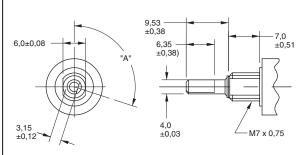
Metric standard dimensions for the shaft and bushing are shown in the drawing. Other dimensions approximately the same as shown in dimensional drawing. Contact Grayhill for exact dimensions. See Style "E" in the Choices and Limitations chart.
