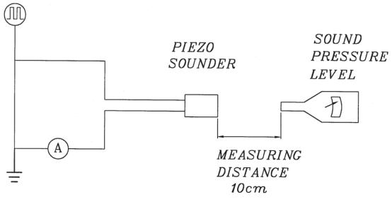
S.P.L. Measuring Circuit Input signal: 10 V p-p, square wave, 800 Hz Mic: RION S.P.L. meter UC30 or equivalent
