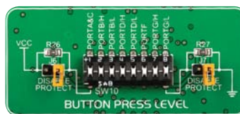
Figure 6-5: Button press level DIP switch (tri-state)
