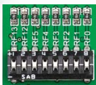
Figure 6-2: Tri-state DIP switch on PORTF
