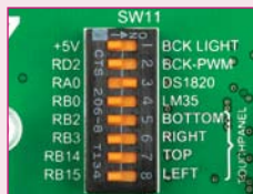
Figure 20-3: Enabled SW11.3 DIP switch
