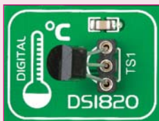
Figure 20-2: DS1820 correctly placed in socket
