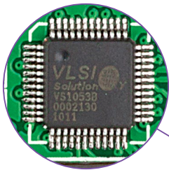
Figure 8-1: On-board VS1053 MP3 codec
