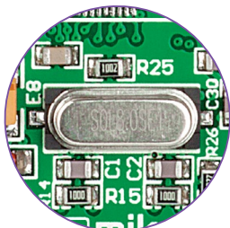
Figure 5-1: Crystal oscillator module (X1)
