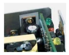
Sil-Pad 400 is a composite of silicone rubber and fiberglass. The material is flame retardant and is specially formulated for use as a thermally conductive insulator. The primary use for Sil-Pad 400 is to electrically isolate power sources from heat sinks.
