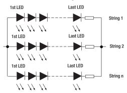
A typical 1W high brightness white LED has a forward voltage of around 3.3V at its operating temperature and draws 350mA. Thus each LED actually draws about 1.15W. Similarly, 3W white LEDs have usually the same forward voltage but can be run at 700mA or more. Using the LED datasheet specification, the optimum LED arrangement and the best driver for each application can be worked out.
