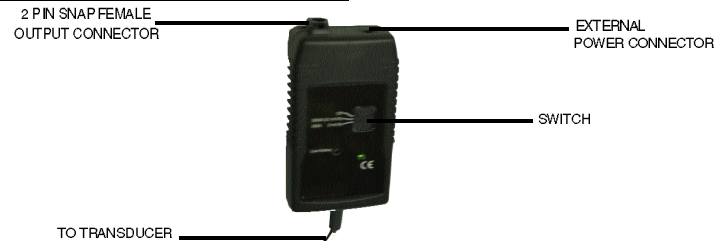
Fig. 1 - ACF-3000DM ELECTRONICS PACKAGE
