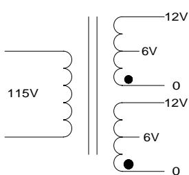
\* Secondary windings are designed to be connected in series or parallel. Windings are not intended to be used independently.
