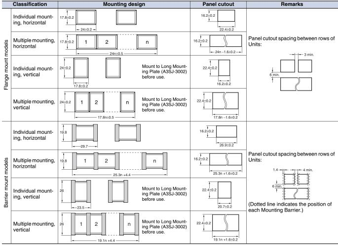
Note: If the panel is to be finished (e.g., coated), make sure that the panel meets the specified dimensions after the coating.
