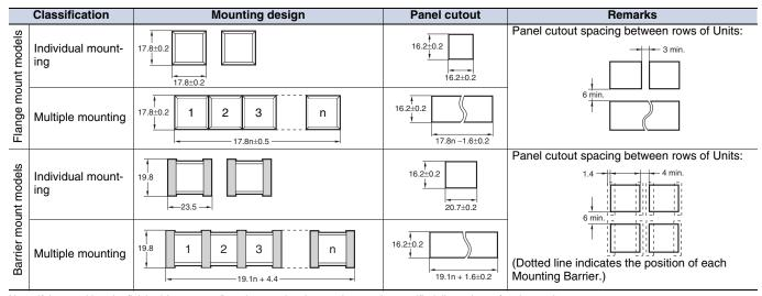
Note: If the panel is to be finished (e.g., coated), make sure that the panel meets the specified dimensions after the coating.
