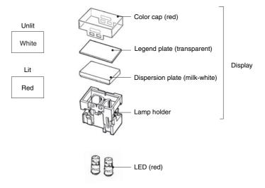
With colored illumination models, the Display surface is white when the LED is not lit and colored when it is lit.
