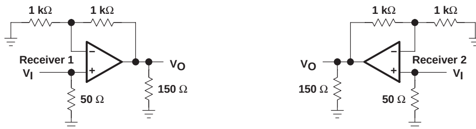
Figure 2. Receiver Input-to-Output Crosstalk Test Circuit
