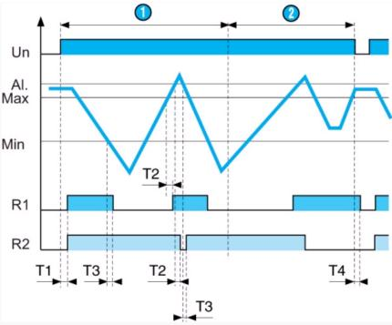
On power-up, probes Min, Max are submerged and probe Al. is above the level of the liquid. Relays R1 and R2 are energised and the pump is ON: emptying starts, the LED for relay R1 is lit. When the Min probe emerges, relay R1 de-energises and the pump if OFF: emptying stops, the LED for relay R1 goes off. If, in the event of a fault, the level continues to rise and reaches proble Al., relay R2 de-energises and the alarm is triggered: the LED for relay R2 is lit.
