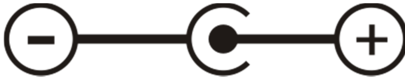
Figure 3 Barrel Connector J7 Polarity
