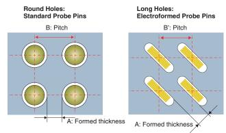
Round hole pitch B > Long hole pitch B' Round hole formed thickness A = Long hole formed thickness A
