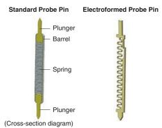
Separating the spring and relay achieves a stable resistance and greater durability.
