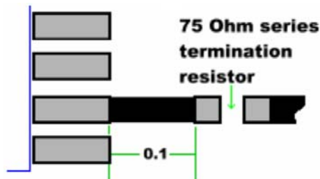
Figure 4. 75\Omega Series Resistor 0.1 Inches from Pin
