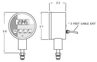
\* Models JVB, JVE, JVR, JVX, JVV No cable for battery powered Model JVW
