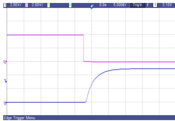
Fig. 68 AVO75-48S05 typical start-up from CNT on
