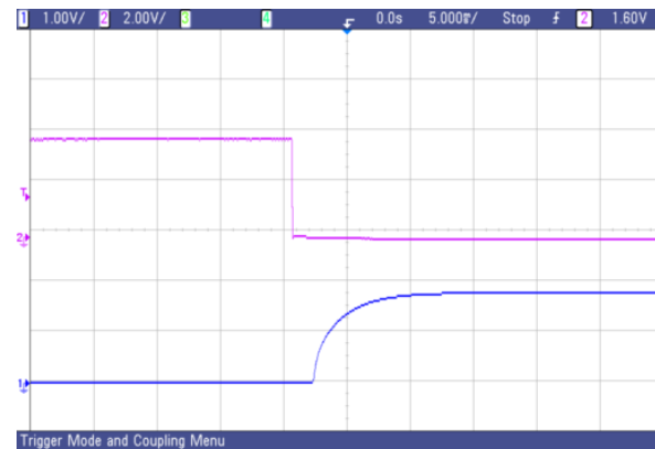
Fig. 62 AVO75-48S1V8 typical start-up from CNT on
