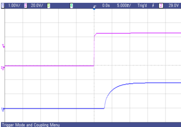
Fig. 61 AVO75-48S1V8 typical start-up from power on
