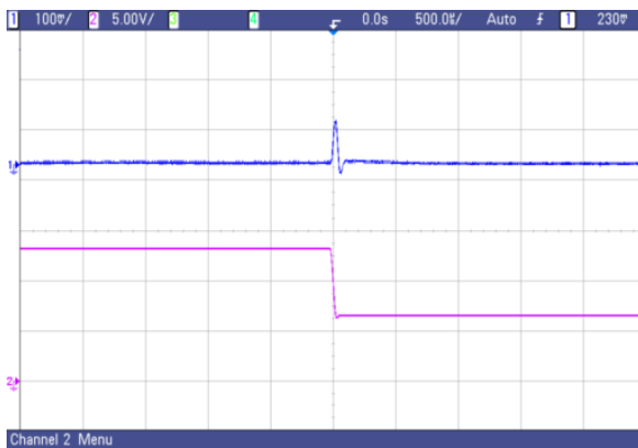
Fig. 42 AVO75-48S05 typical transient response to step decrease in load from 50% to 25% of full load, room temperature, 48Vdc input ( \Delta I_o/\Delta t=0.1A/1\mu s )
