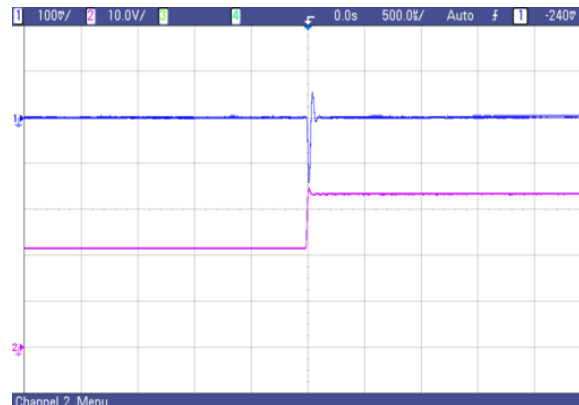
Fig. 37 AVO75-48S2V5 typical transient response to step increase in load from 50% to 75% of full load, room temperature, 48Vdc input ( \Delta I_o/\Delta t=1A/1\mu s )
